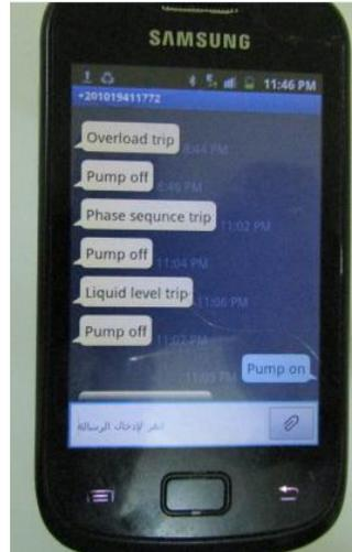
Fig.12. shows the SMS sent by the user to control system to remotely ON/OFF the pump and the replied SMS (confirmation message) from the control system to the user.
