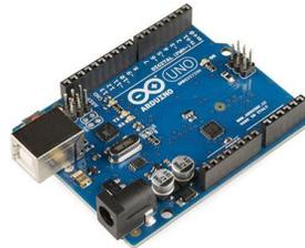
Fig.4. Arduino Uno board
