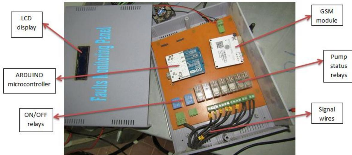
Fig.10.hardware setup of the performed system.
