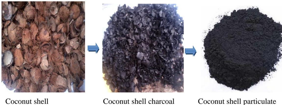
Plate 1. Production process products: coconut shell – coconut shell particulate
